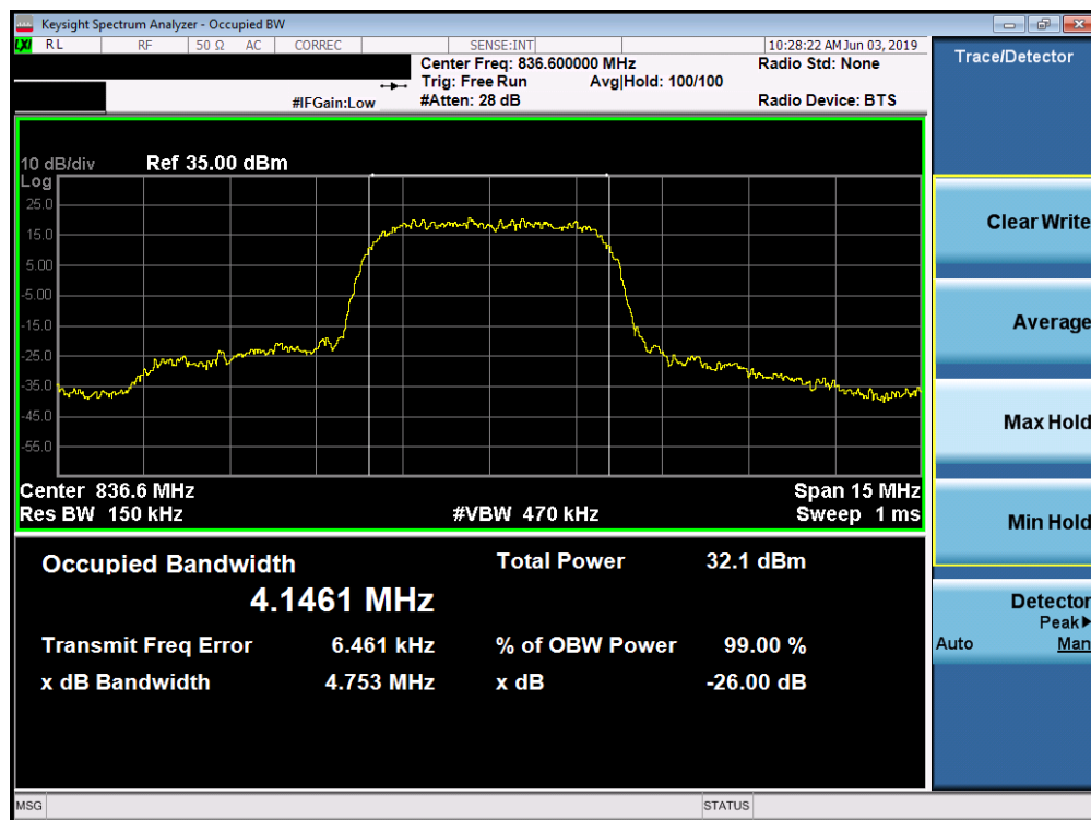
Plot 7-5. Occupied Bandwidth Plot (Cellular WCDMA Mode)
