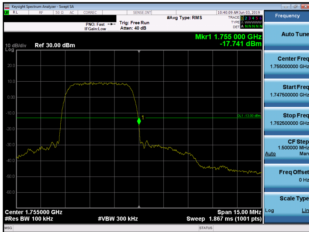
Plot 7-60. Band Edge Plot (AWS WCDMA Mode - High Channel)
