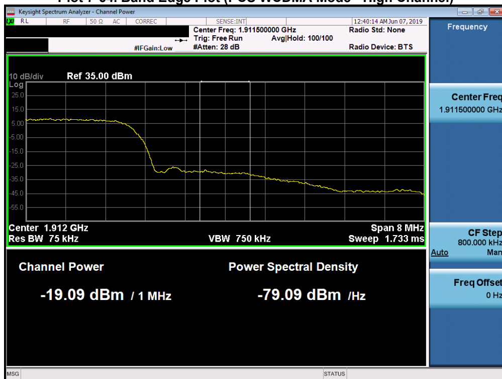
Plot 7-65. 4MHz Span Plot (PCS WCDMA Mode - High Channel)
