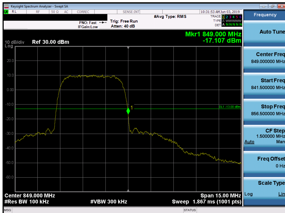
Plot 7-57. Band Edge Plot (Cellular WCDMA Mode - High Channel)
