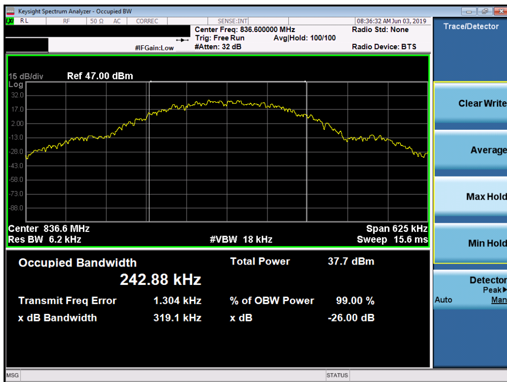
Plot 7-1. Occupied Bandwidth Plot (Cellular GPRS Mode)
