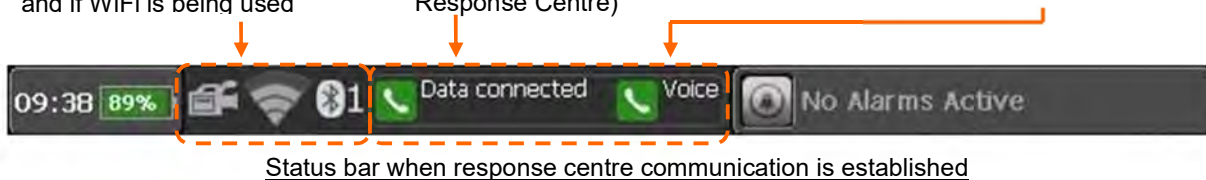
Status bar when response centre communication is established
