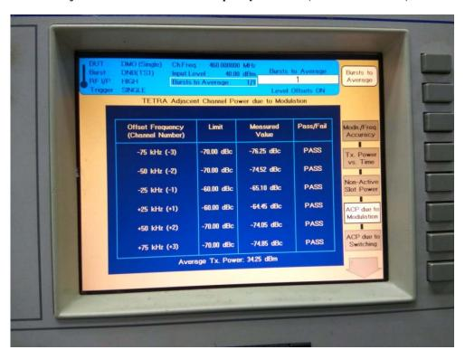
Adjacent Channel Power for Frequency 469.9875 MHz (Modulation: DMO)
