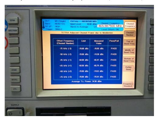
Adjacent Channel Power for Frequency 450.0125 MHz (Modulation: DMO)
