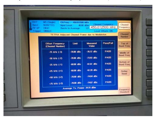
Adjacent Channel Power for Frequency 460 MHz (Modulation: TMO)
