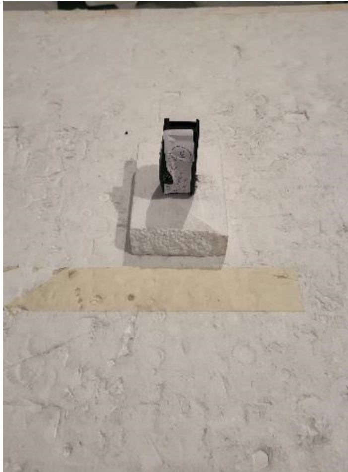
Figure 1. Radiated Emissions Test Setup, Front
