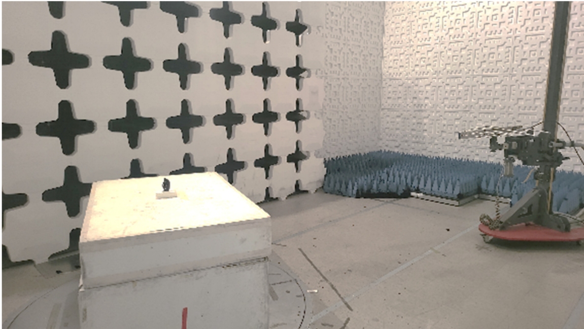
Figure 4. Radiated Emissions Test Setup, 200 MHz to 1GHz, Back
