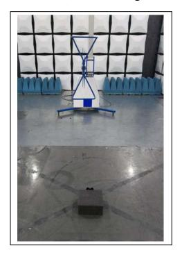
Radiated Spurious, Less Than 30 MHz
