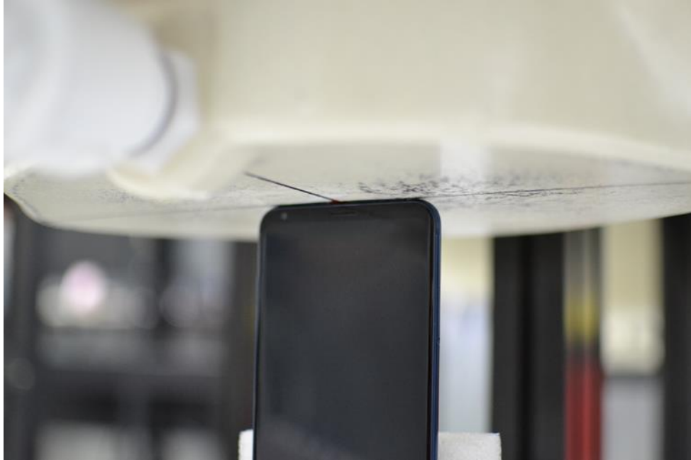
SAR Test Setup Photo 13: Top at 0.0 cm
