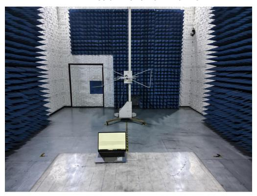
RADIATED EMISSION TEST SETUP ABOVE 1GHz
