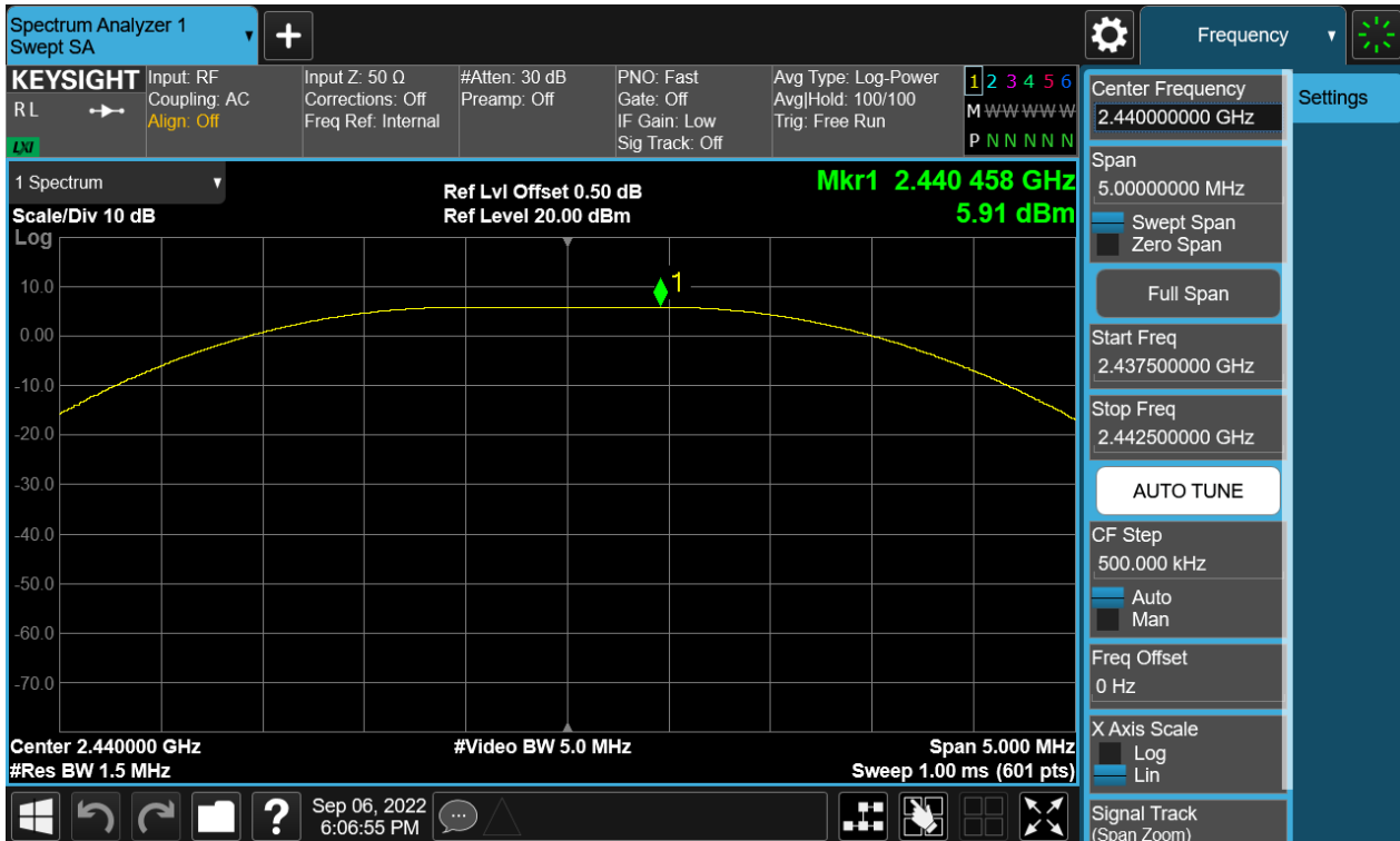
Figure 6: The plots of Peak Conducted Output Power, BLE-2M, 2480MHz
