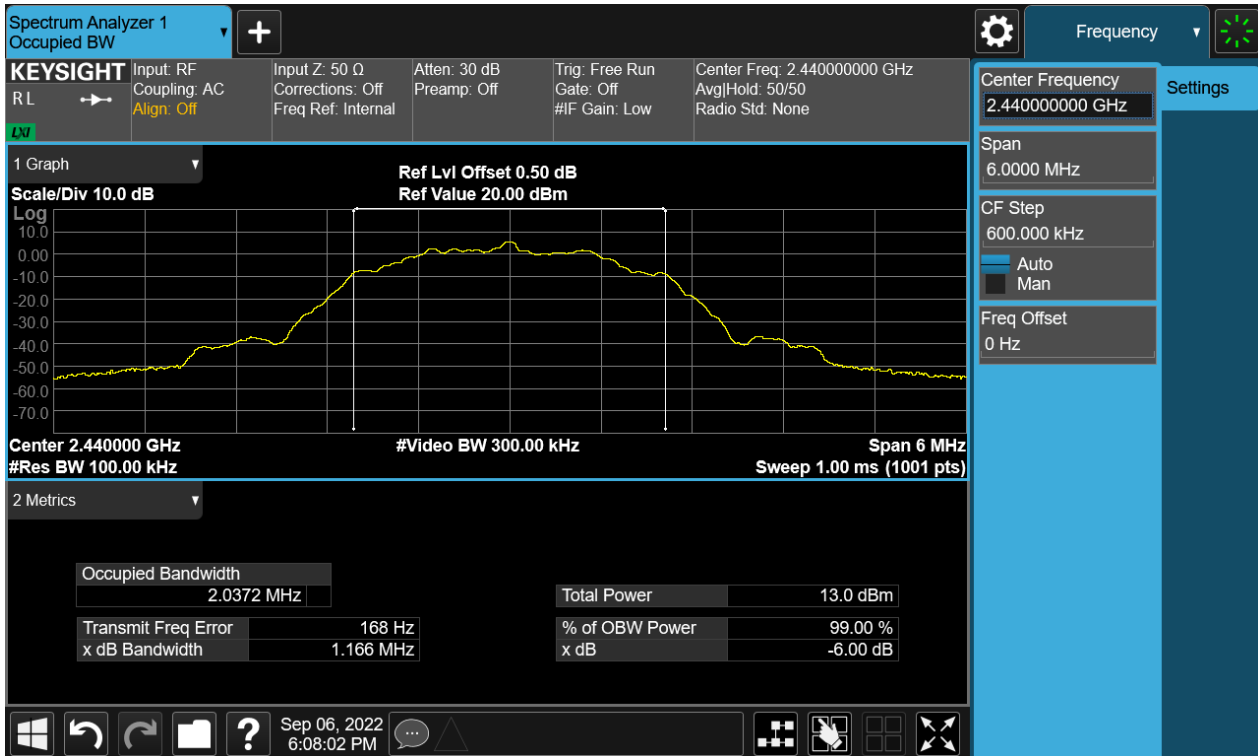
Figure 16: The plots of 99% Bandwidth, BLE-2M, 2440MHz
