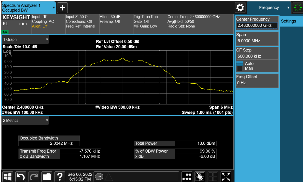
Figure 18: The plots of 99% Bandwidth, BLE-2M, 2480MHz
