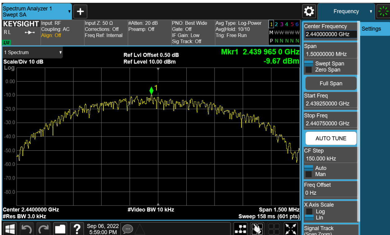
Figure 20: The plots of Power Spectral Density, BLE-1M, 2440MHz
