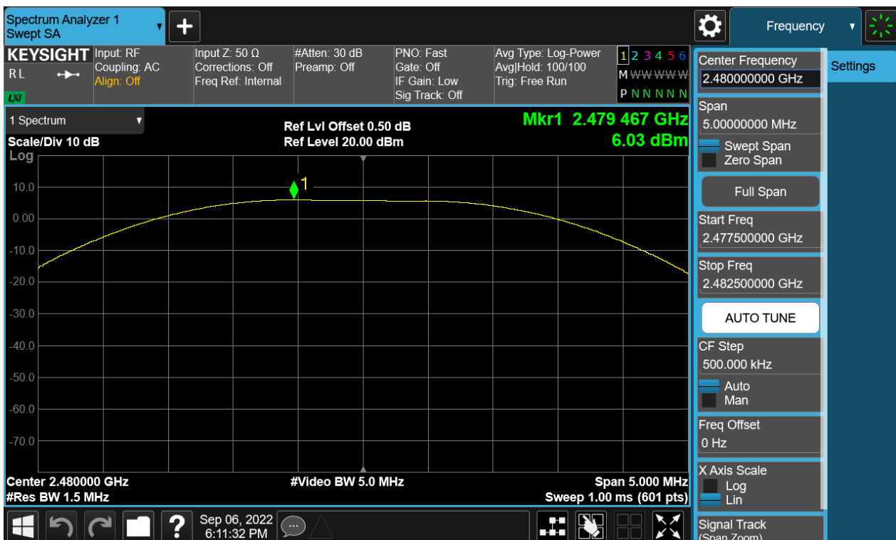
Figure 6: The plots of Peak Conducted Output Power, BLE-2M, 2480MHz
