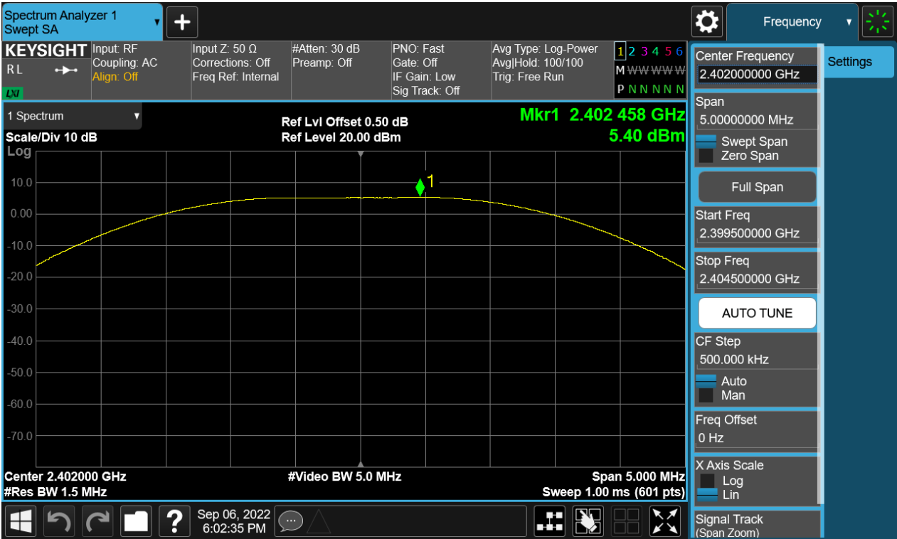
Figure 4: The plots of Peak Conducted Output Power, BLE-2M, 2402MHz
