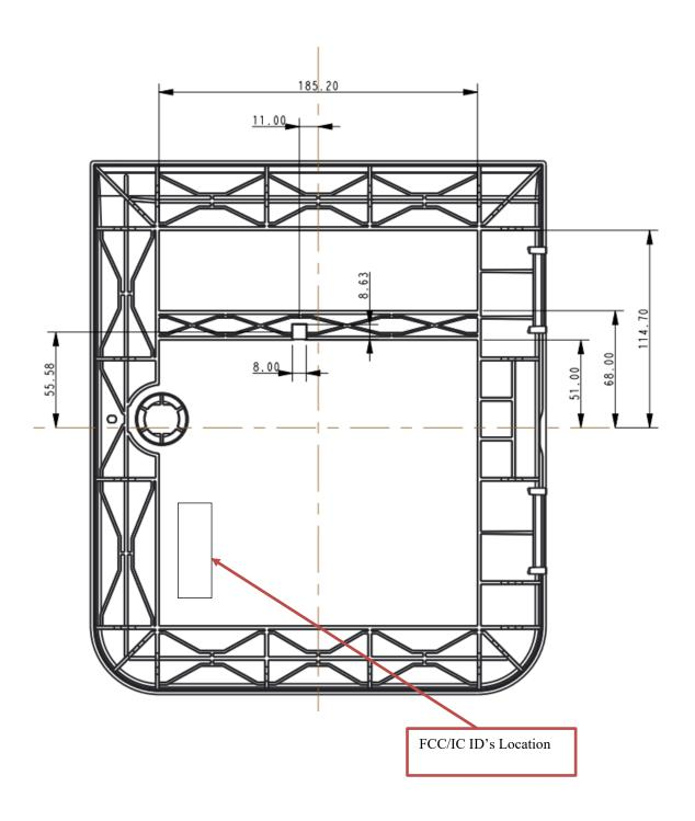
For Quicksilver 7" All-In-One, label is to be placed by the installer on the rear of the wall-mounting plate in the location shown:
