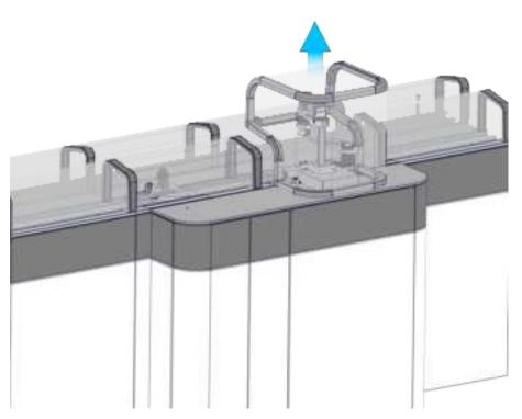
Pull up the Decapper head and rotate it to the decap position by hand.
