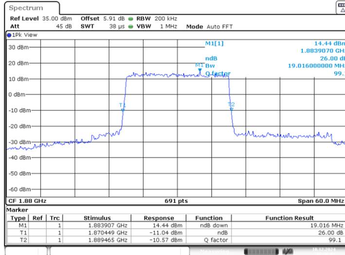
**LTE band 2 , 20MHz Bandwidth,MID,16QAM (-26dBc BW)**
