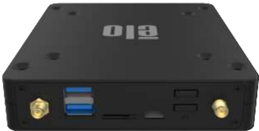
Wi-Fi and BT Antenna USB 3.0 microSD GPIO Home Power Wi-Fi Antenna
