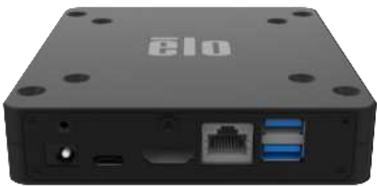
DC In Type C HDMI Ethernet USB 3.0
