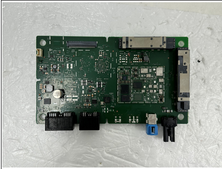
Bottom view of Main PCB
