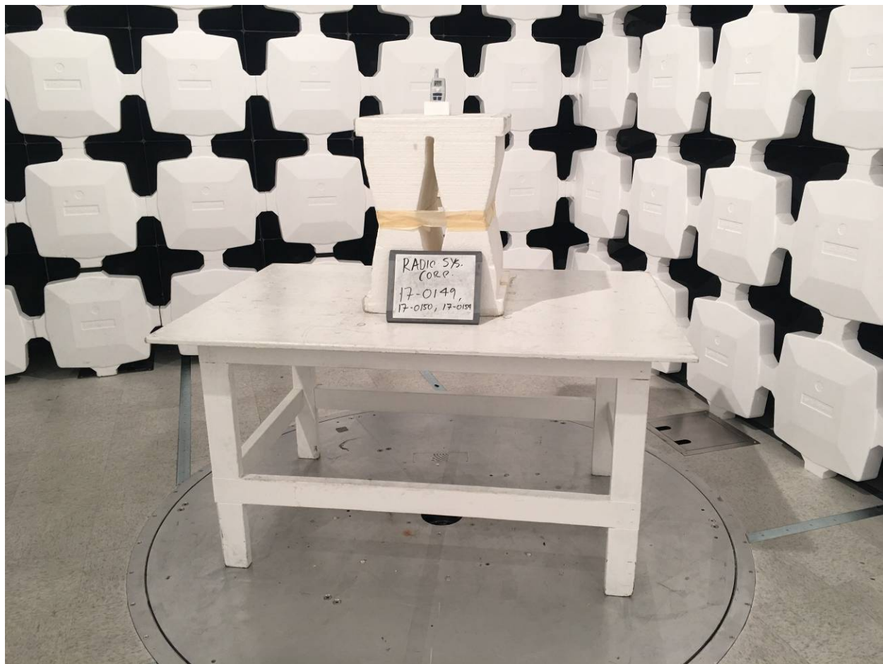
Figure 5. Radiated Emissions Test Setup, above 1 GHz, Close-up
