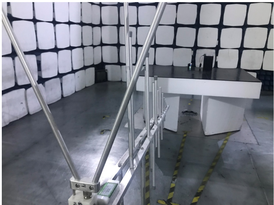
Radiation Emission Test Setup (30MHz to 1GHz)
