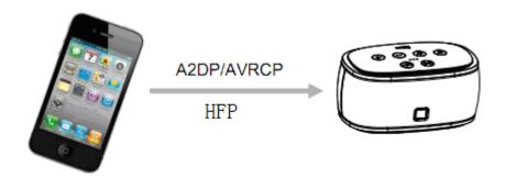
A, Slide the switch to "Bluetooth "side, the unit enters into pairing mode automatically (blue and red LED flashes alternately.)
