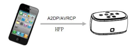
A, Slide the switch to "Bluetooth "side, 10 seconds later, the unit will connect with the last connected mobile phone.
