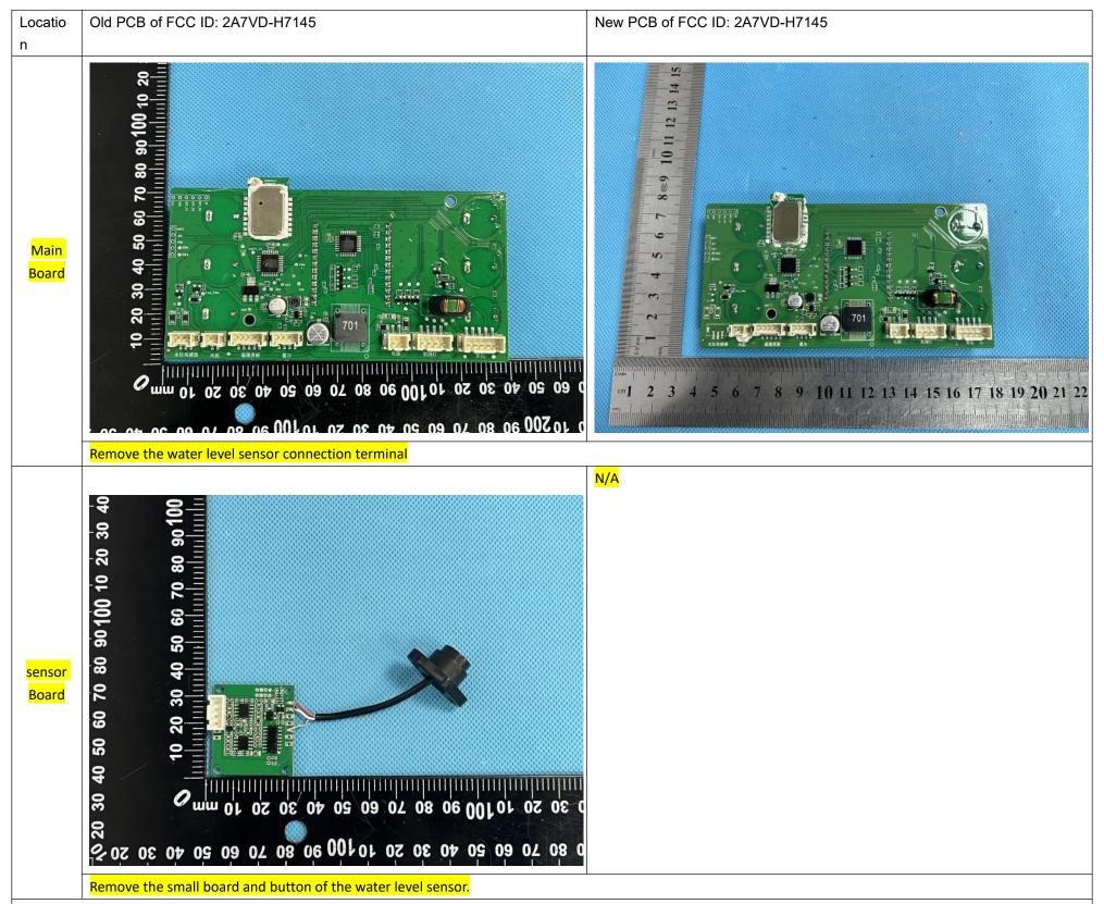
Modifications that do not change the fundamental RF characteristics and that do not degrade the unwanted emissions of the certified product, please refer to test report for more details; We attach new photographs to identify the modified product.
