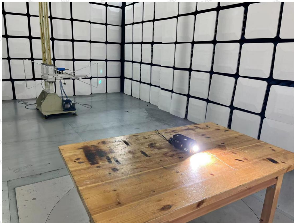
Photo of Radiation Emission Test
