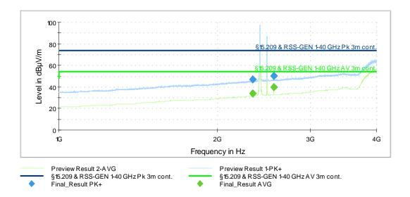
The emissions @ 2.405 MHz is the wanted IEEE802.15.4 signal The emissions @ 2.480 MHz is the wanted BLE signal The emissions @4 GHz is the wanted UWB signal
