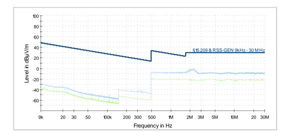
All emissions are more the 20 dB from the limit, so no final measurement was performed.
