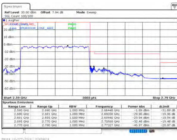
n41 SCS=30kHz DFT_BPSK BW=80MHz HighChannel=529998 RB=216@0
