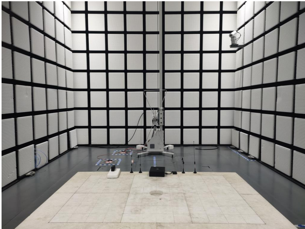
Fig. 2 Radiated emission setup photo(30MHz-1GHz)
