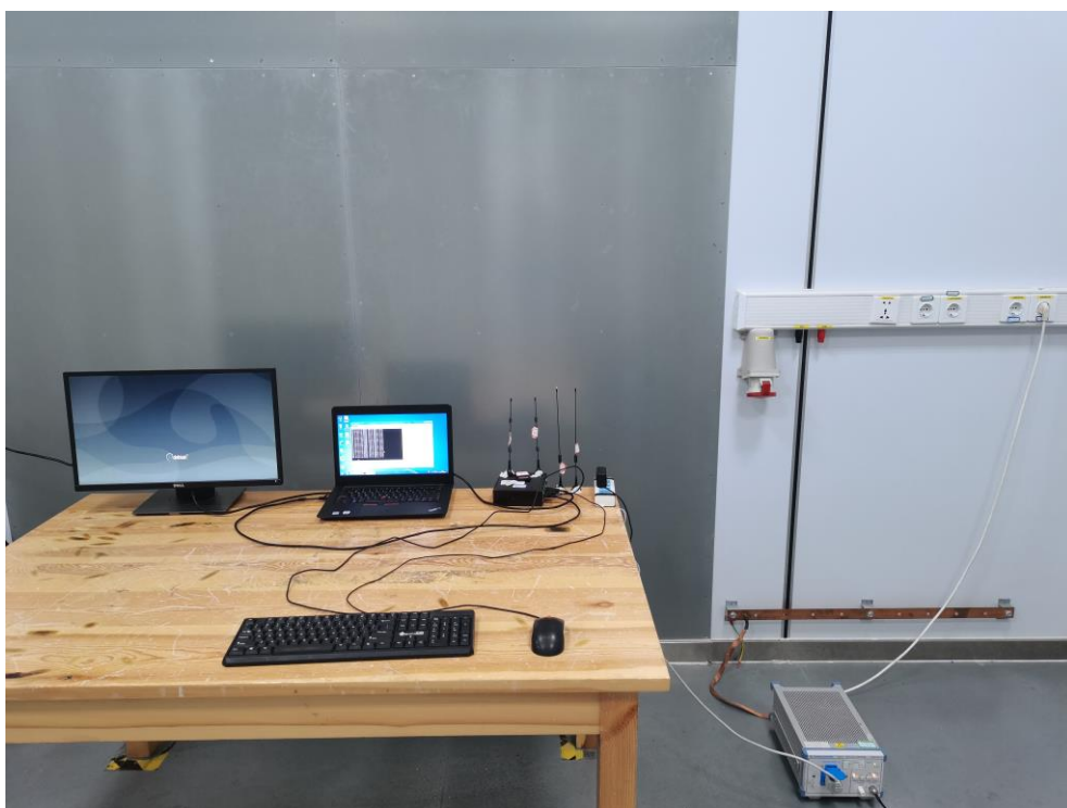
Fig. 4 Power line conducted emission setup photo
