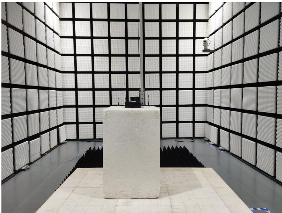
Fig. 3 Radiated emission setup photo(Above 1GHz)
