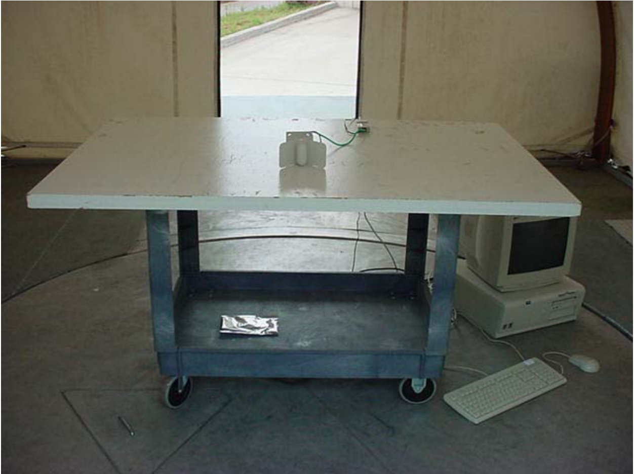
Figure 1: Mobile Mark SCR14-5725CT - 14dBi Corner Reflector
