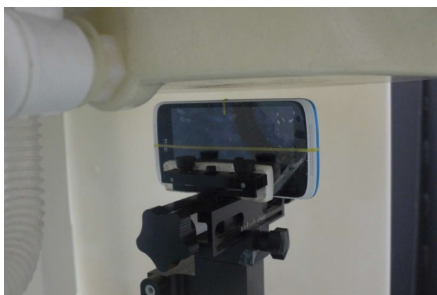
Left Side, Test Separation 1 cm
