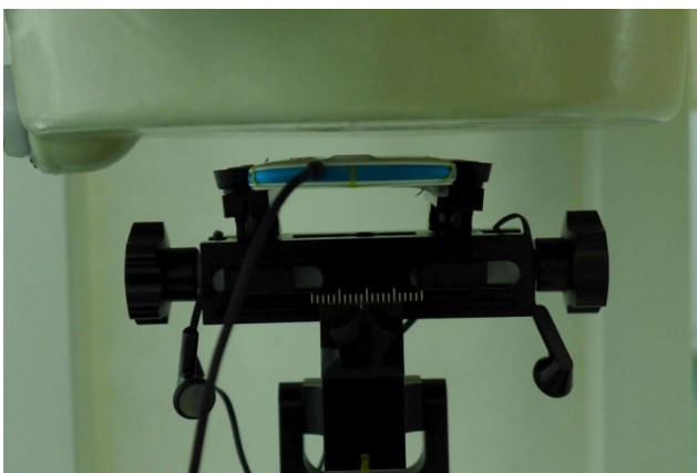
Back with Headset, Test Separation 1 cm
