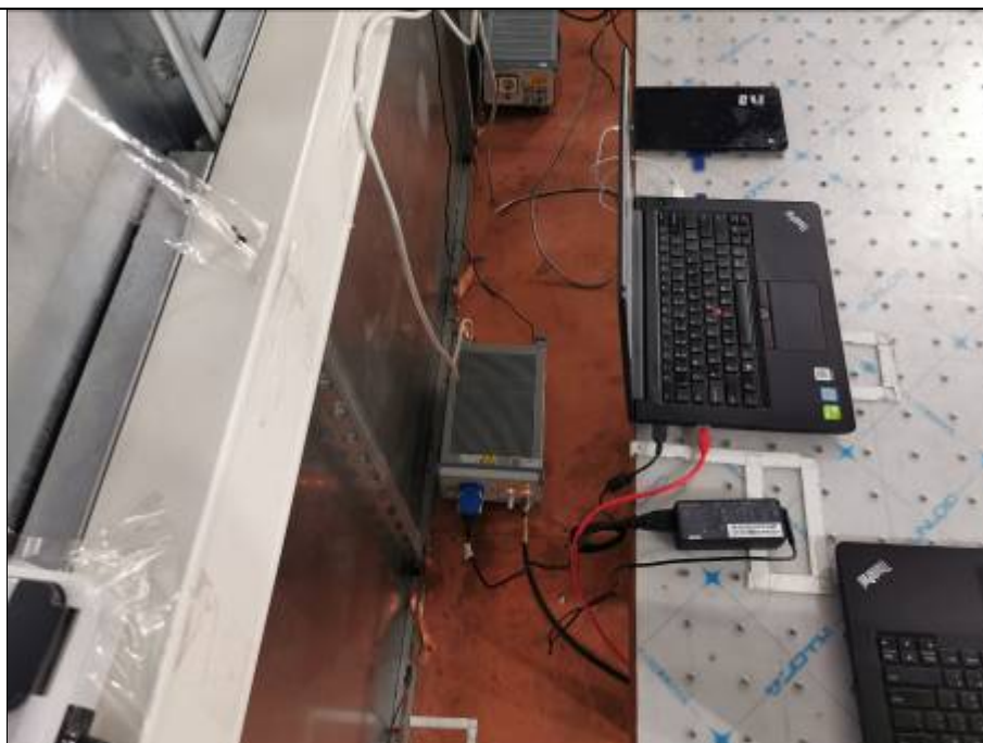
Conducted Emissions Test Setup (with laptop)
