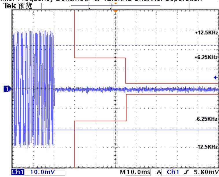
Transmitter Frequency Behaviour @ 12.5kHz Channel Separation-----On – Off
