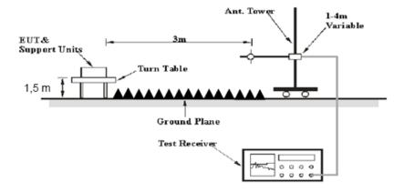
The radiated emission below 1GHz tests were performed in the 10 meters chamber test site, above 1GHz tests were performed in the 3 meters chamber test site B, using the setup accordance with the ANSI C63.10-2013. The specification used was the FCC 15.209, and FCC 15.247 limits.
