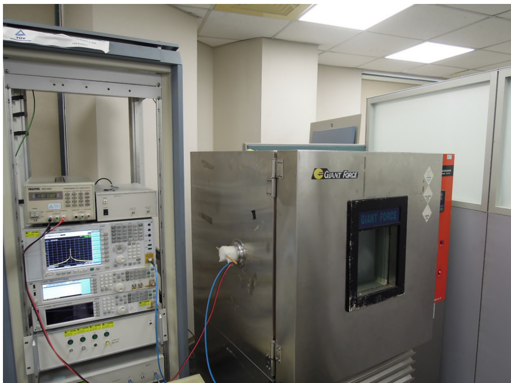
Photograph 4: Set-up for for Conducted testing
