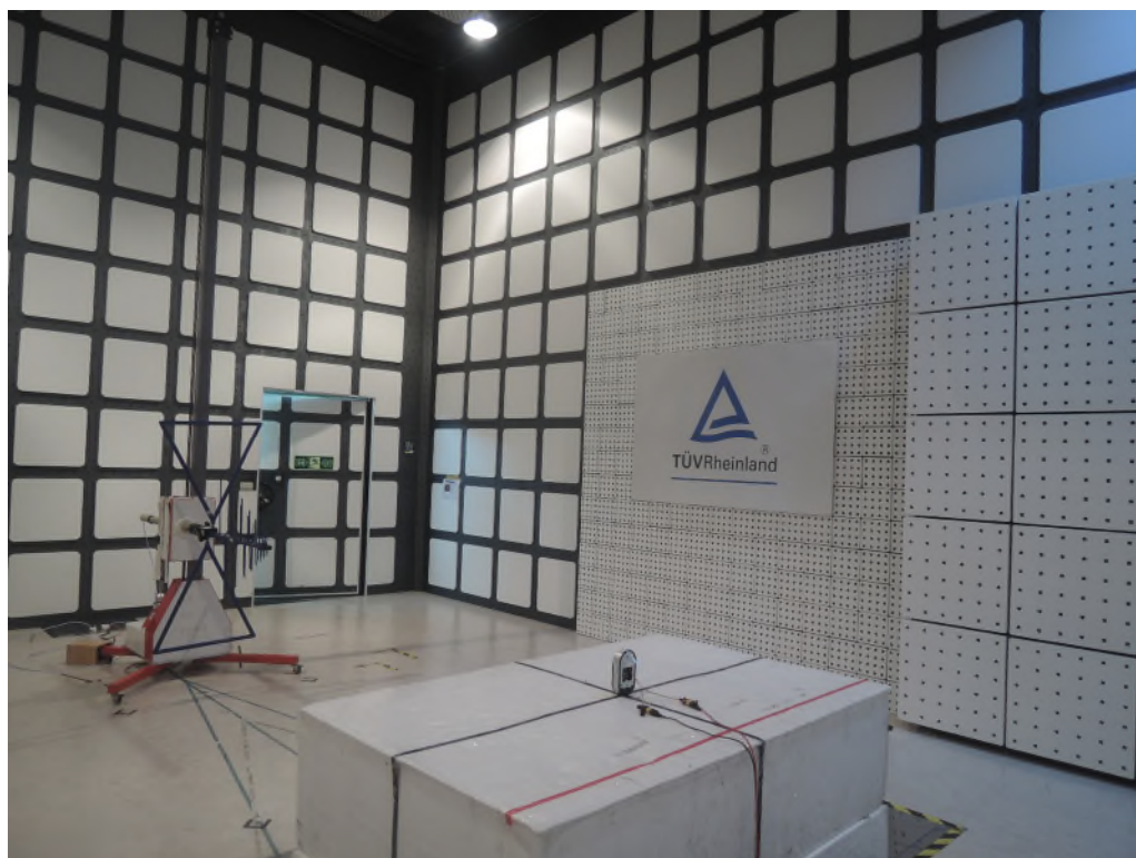
Photograph 2: Set-up for Radiated Emissions (Back View 1)
