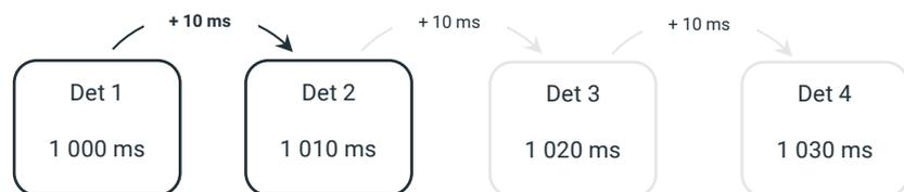
If 2 is selected as an **Interval number**, the PU will suggest a delay matching the increment entered between the 1<sup>st</sup> and 2<sup>nd</sup> detonator for the 3<sup>rd</sup> detonator. The delay for the 4<sup>th</sup> detonator will then match the increment entered between the 2<sup>nd</sup> and the 3<sup>rd</sup> detonator.
