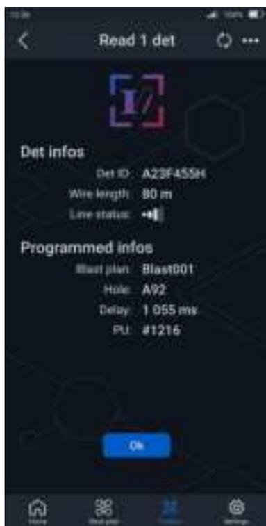
This test allows to read the information stored in a connected detonator. Depending on its status (programmed or not) different levels of information will be available.
