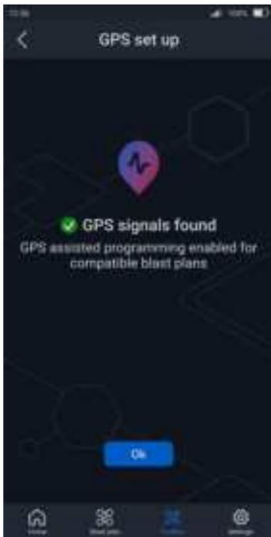
This setup functionality enables the PU to collect GPS signals, preparing it for GPS-assisted programming
