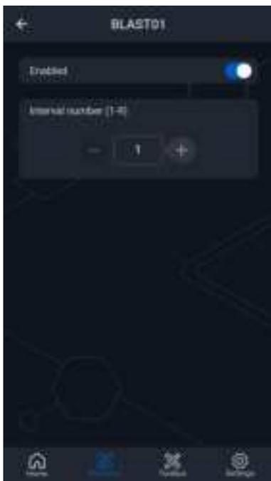
The **Delay pattern** function gives an assistance for manual programming. After programming a couple of detonators, the PU will suggest the next delays according to the chosen **Interval number**.
