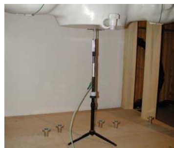
Figure 12.1 Dipole Validation Test Setup
