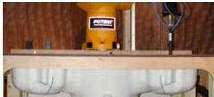
Figure 5.1 SAM Twin Phantom
