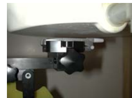
Figure 14.10 Body SAR Test Setup -- w/o Holster --
