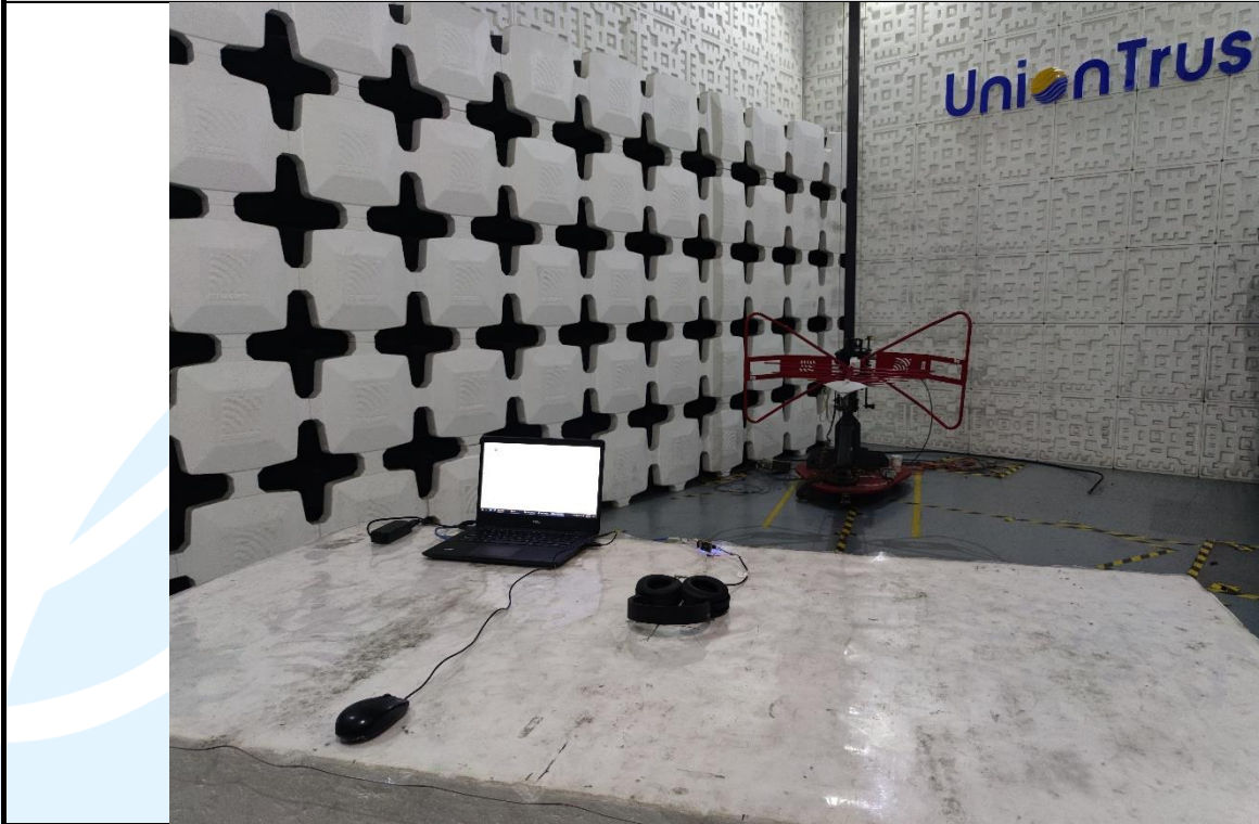
Radiated emission Test Setup (30 MHz~1 GHz)
