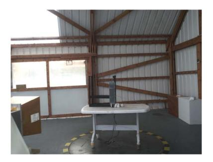
Photograph No.10 Spurious emissions measurement setup at the OATS above 18 GHz
