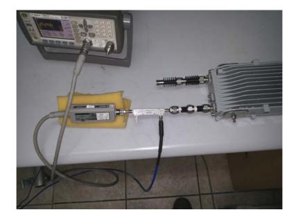
Photograph No.4 Conducted spurious emissions measurement setup
