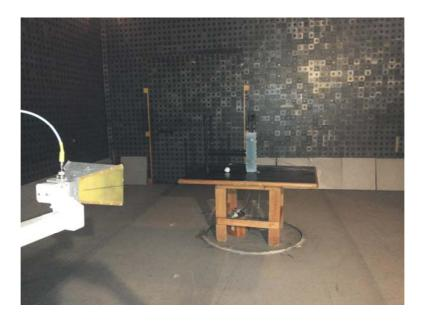
Photograph No.8 Spurious emissions measurement setup in the anechoic chamber, EUT close view
