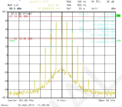
FCC Part 22 Occupied Bandwidth, 161.65 MHz, 4FSK mode, High Power
