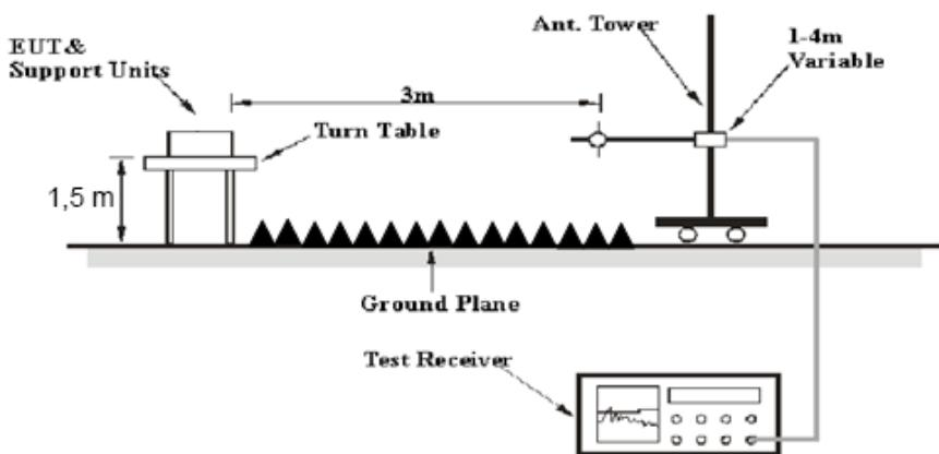
The radiated emission below 1GHz tests were performed in the 3 meters chamber test site A, above 1GHz tests were performed in the 3 meters chamber test site B, using the setup accordance with the ANSI C63.10-2013. The specification used was the FCC 15.209, and FCC 15.247 and the RSS-247 Clause 5.5, RSS-GEN Clause 8.10 limits.
