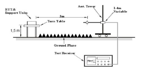
The radiated emission below 1GHz tests were performed in the 3 meters chamber test site A, above 1GHz tests were performed in the 3 meters chamber test site B, using the setup accordance with the ANSI C63.10-2013. The specification used was the FCC 15.209, and FCC 15.247 and the RSS-247 Clause 5.5, RSS-GEN Clause 8.10 limits.
