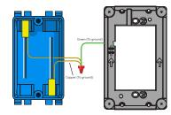
6 Install the mounting plate to the wall box and pull the rest of the wires through the mounting plate.
