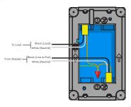
7 Identify and connect the wires to the back of the switch. Insert the wire into the terminal and secure it by hand-tightening the set screw..
