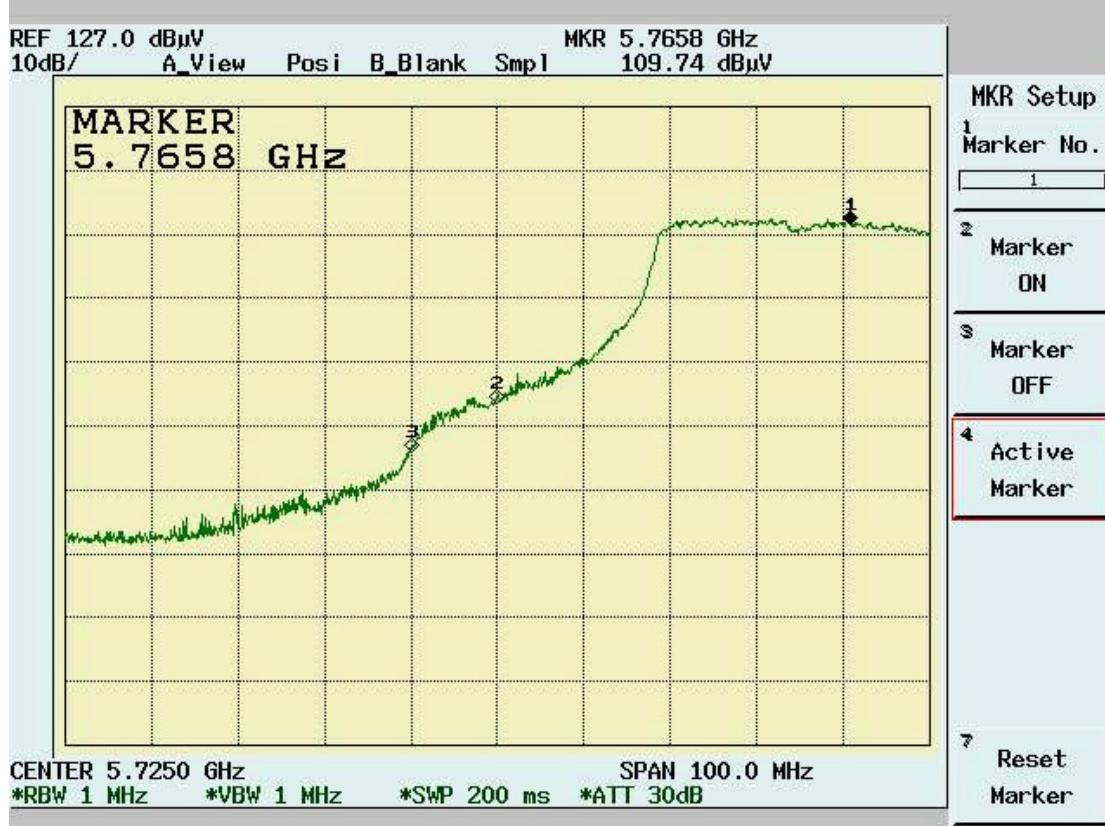
Band Edge Conducted Measurement (Turbo Mode Channel 5)
