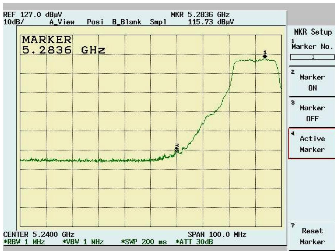
Band Edge Conducted Measurement (Normal Mode Channel 8)
