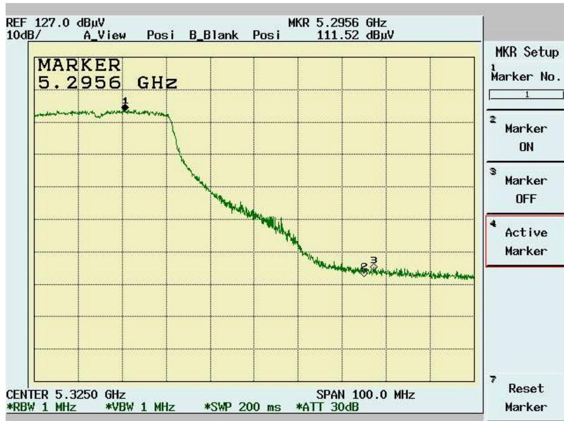
Band Edge Conducted measurement (Turbo Mode Channel 4)
