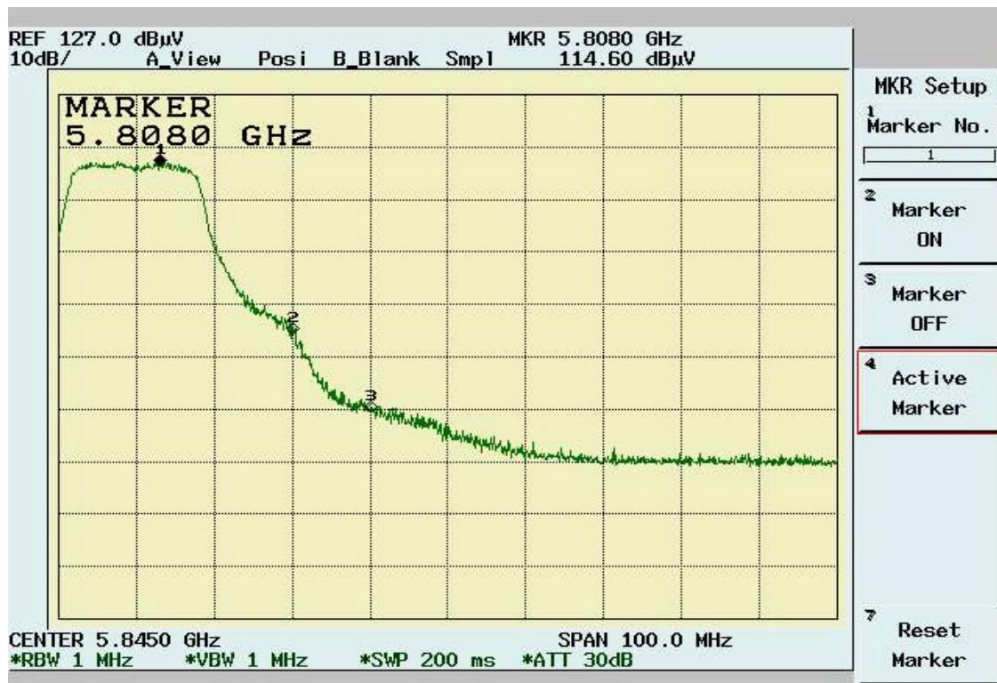
Band Edge Conducted measurement (Normal Mode Channel 9)
