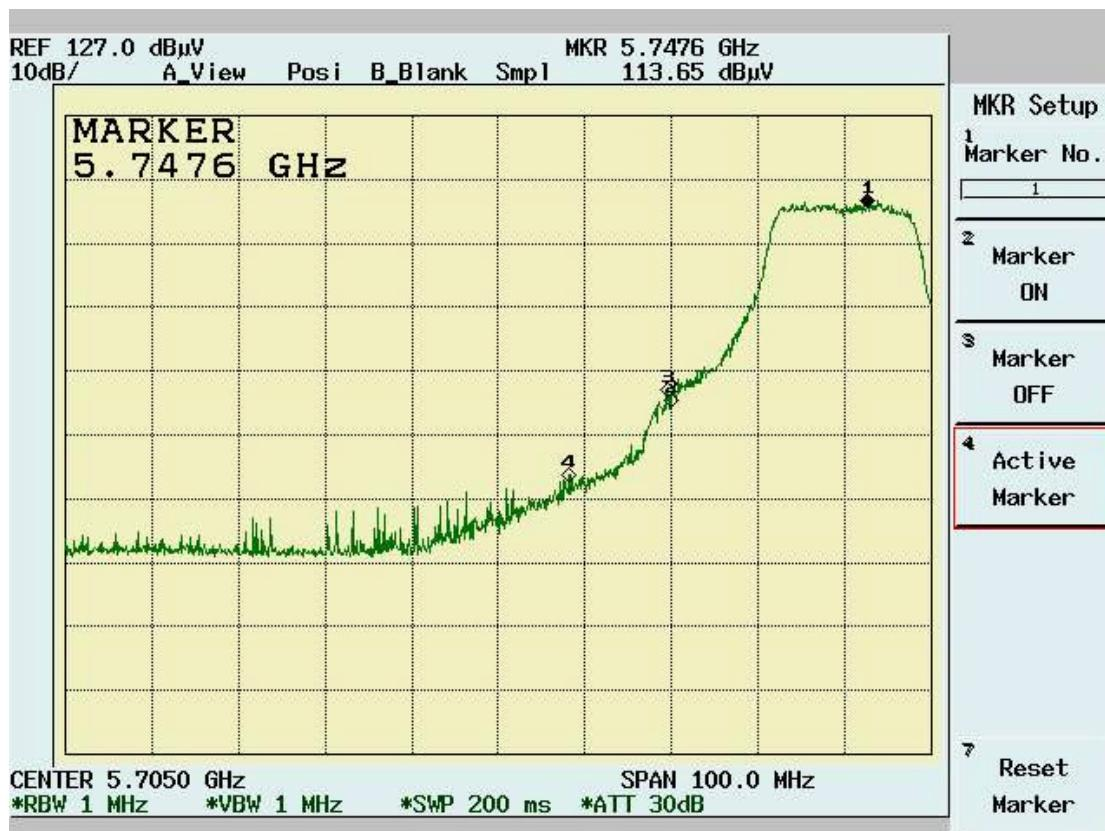
Band Edge Conducted measurement (Turbo Mode Channel 3)
