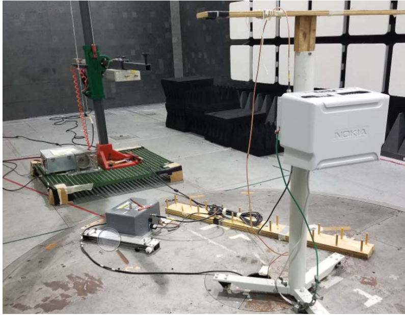
Figure 5. Photo of AC Power Line Conducted Test
