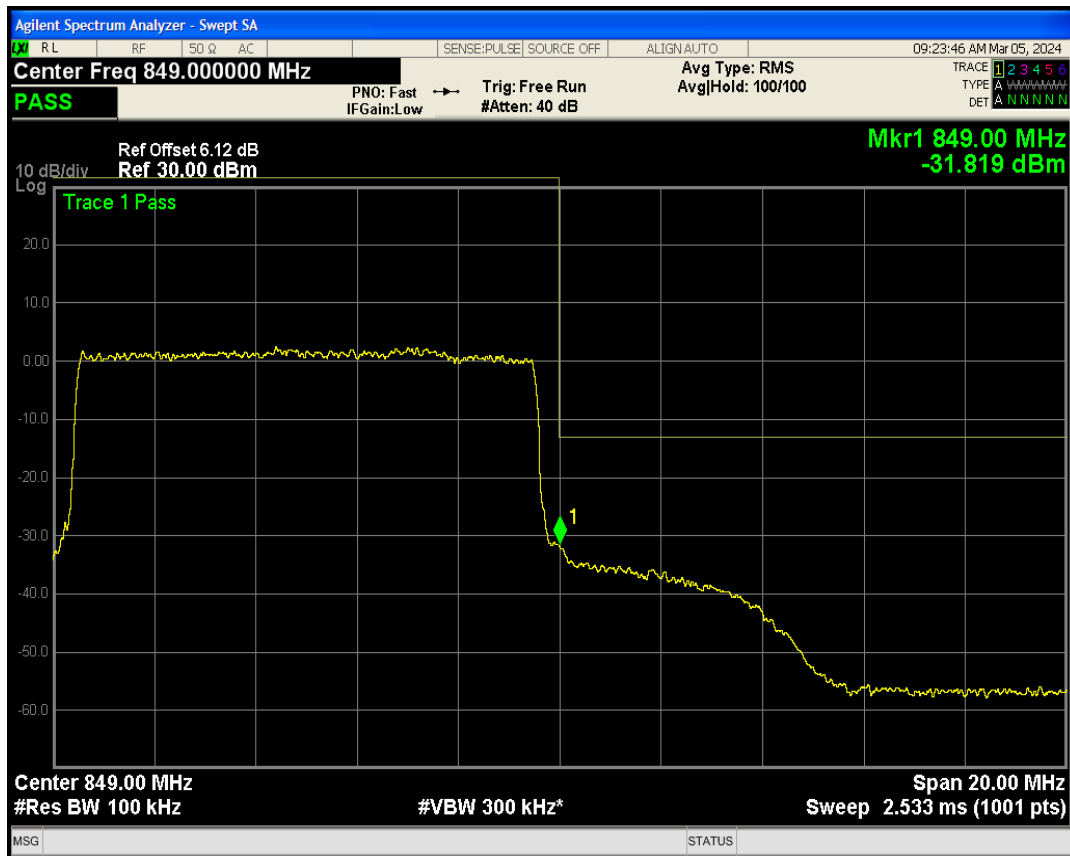
Band7 QPSK BW=5MHz Channel=20775 RB Size=25 Position=#0
