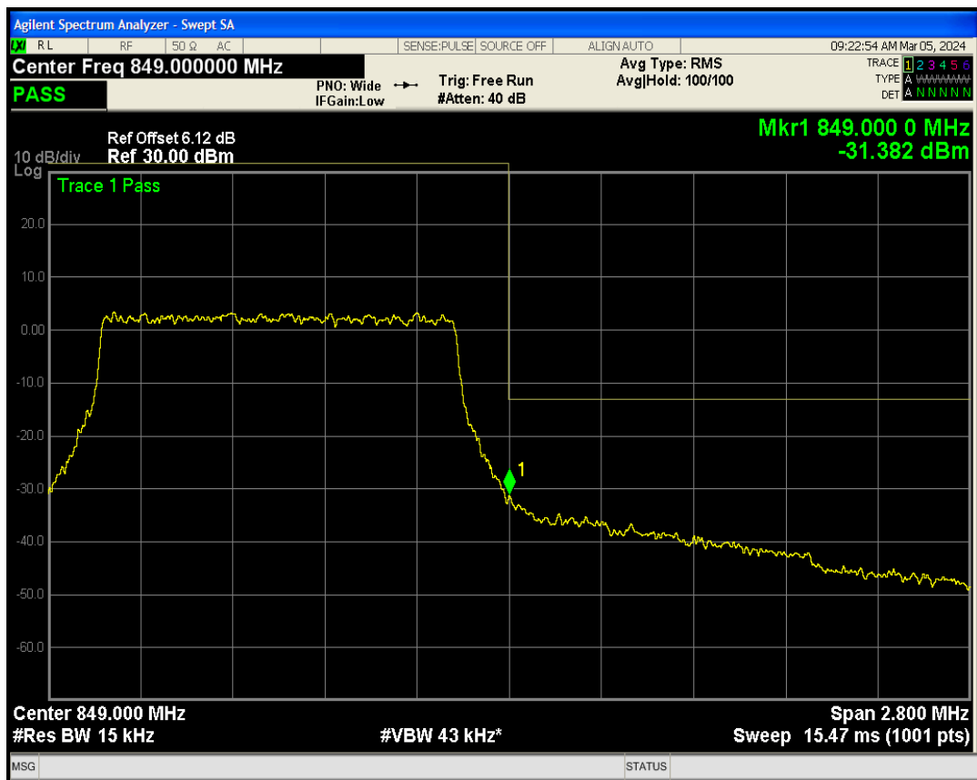
Band5 QPSK BW=3MHz Channel=20415 RB Size=15 Position=#0
