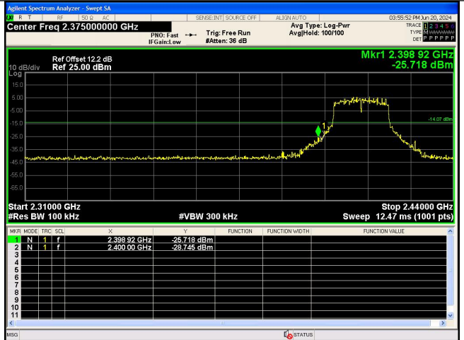
Out Of Band Emission IEEE 802.11g Channel 1 20MHz Antenna 0
