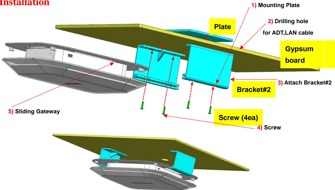
a) Drill 4 holes on the wall or ceiling to align with mounting Plates (1). Refer to the attached diagram.
