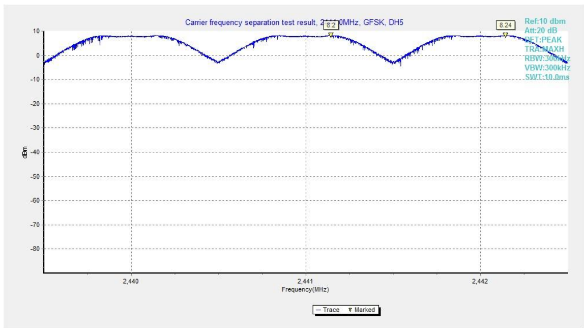
Fig.91. Carrier frequency separation measurement: GFSK, Channel 39
