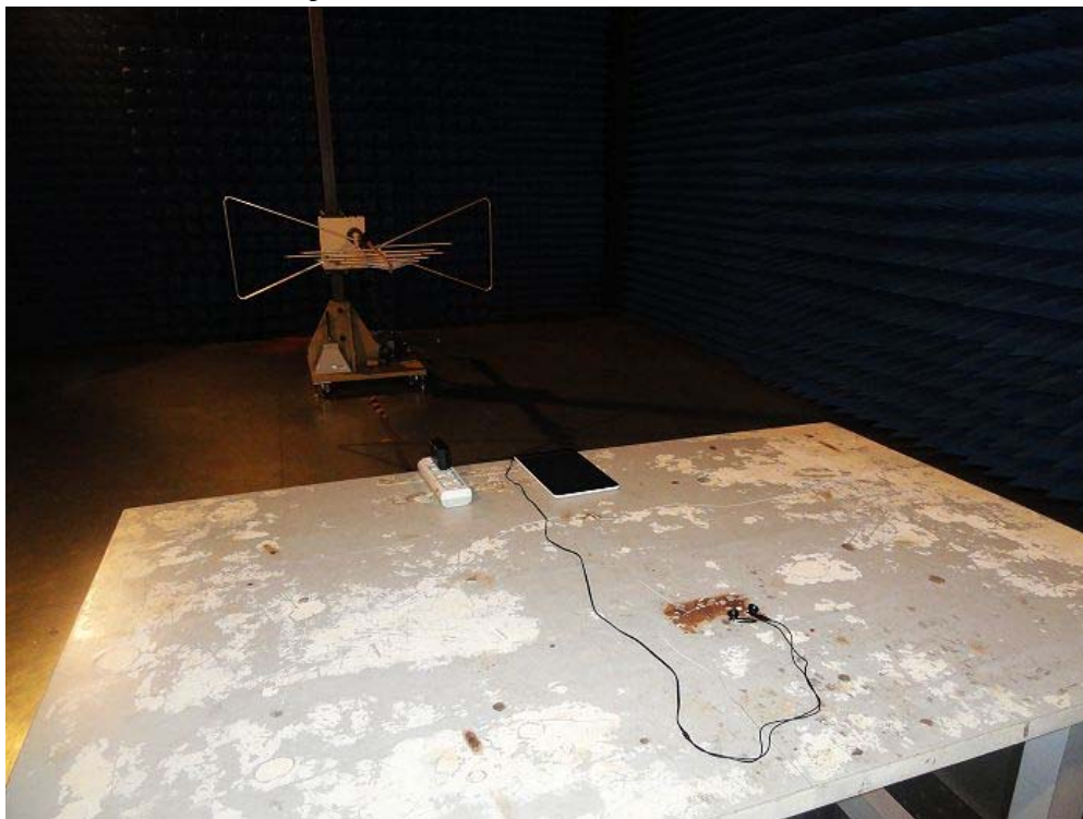
Radiated Emission Test Setup:
