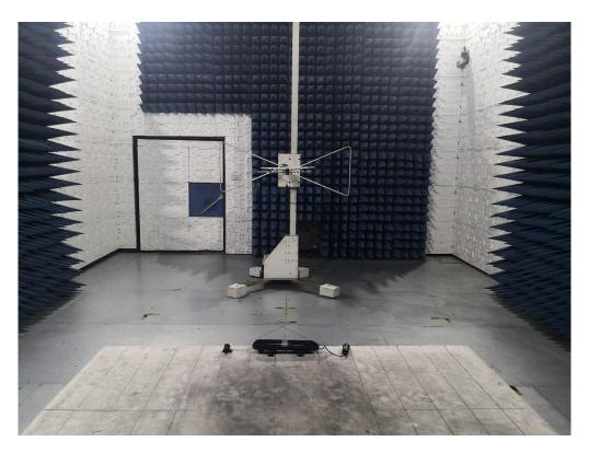
FCC RADIATED EMISSION TEST SETUP ABOVE 1GHZ
