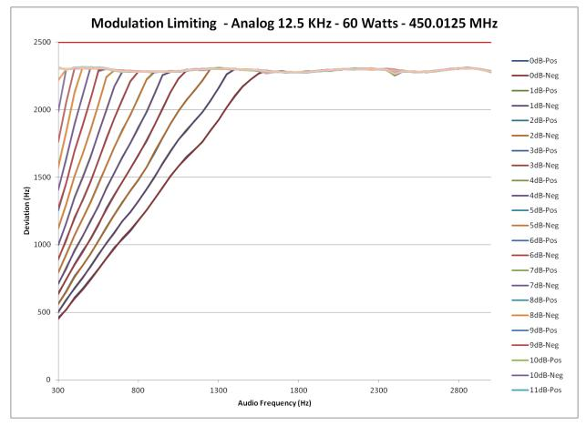
E1-11.11 Audio Modulation Limiting – Modulation Characteristics, 12.5 kHz Channels – 460.0125 MHz
