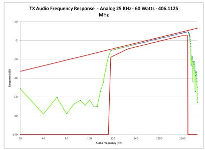
E1-10.1 Audio Frequency Response – Modulation Characteristics, 25 kHz Channels – 406.1125 MHz
