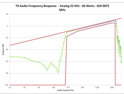
E1-10.3 Audio Frequency Response – Modulation Characteristics, 25 kHz Channels – 429.9875 MHz
