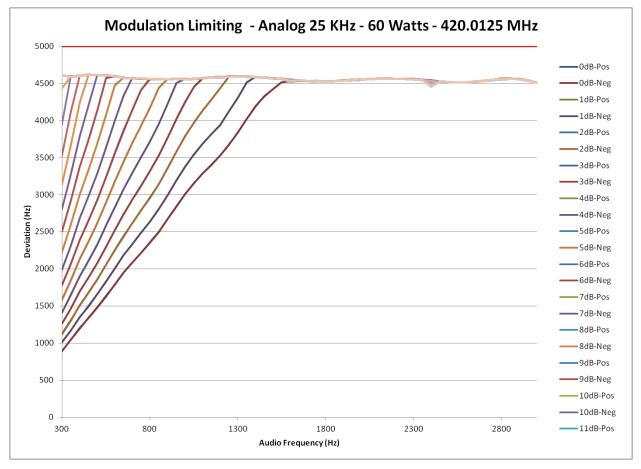
E1-11.3 Audio Modulation Limiting – Modulation Characteristics, 25 kHz Channels – 429.9875 MHz
