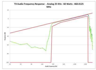
E1-10.5 Audio Frequency Response – Modulation Characteristics, 25 kHz Channels – 460.0125 MHz
