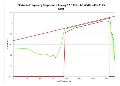
E1-10.7 Audio Frequency Response – Modulation Characteristics, 12.5 kHz Channels – 406.1125 MHz
