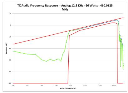
E1-10.11 Audio Frequency Response – Modulation Characteristics, 12.5 kHz Channels – 460.0125 MHz
