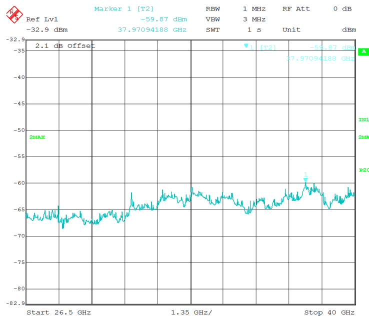
Figure 46: Spurious emission measured from 26.5 GHz to 40 GHz at Ch. 0-Peak
