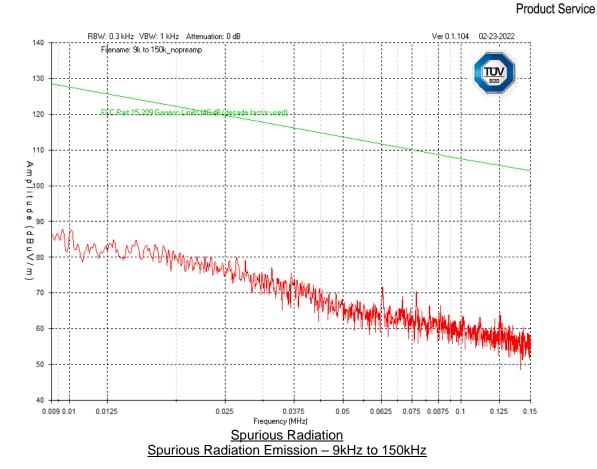
Note: No significant emission (i.e., less than 10dB below the limit) was noted.
