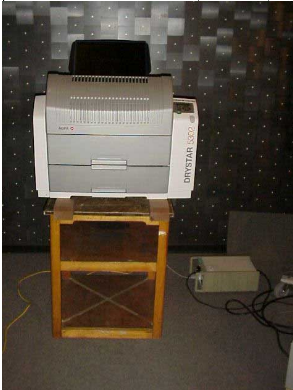
photo 2: conducted emission mains (0.15-30MHz)
