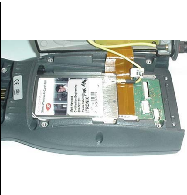
Photograph A.1-3 - AirCard 860 PCMCIA Modem installed in IX100X Rugged Handheld PC
