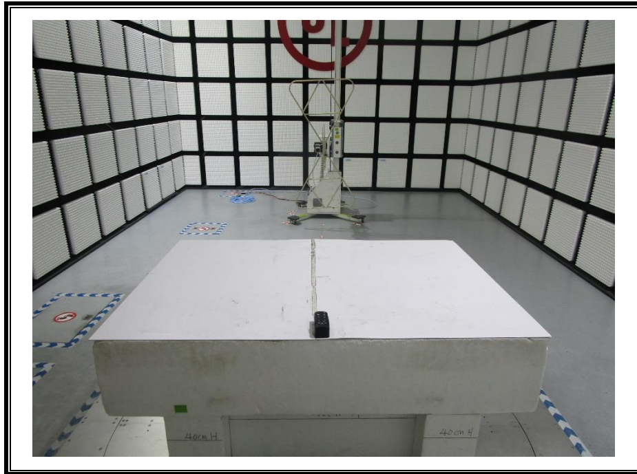
RADIATED RF MEASUREMENT SETUP (Below 30MHz)
