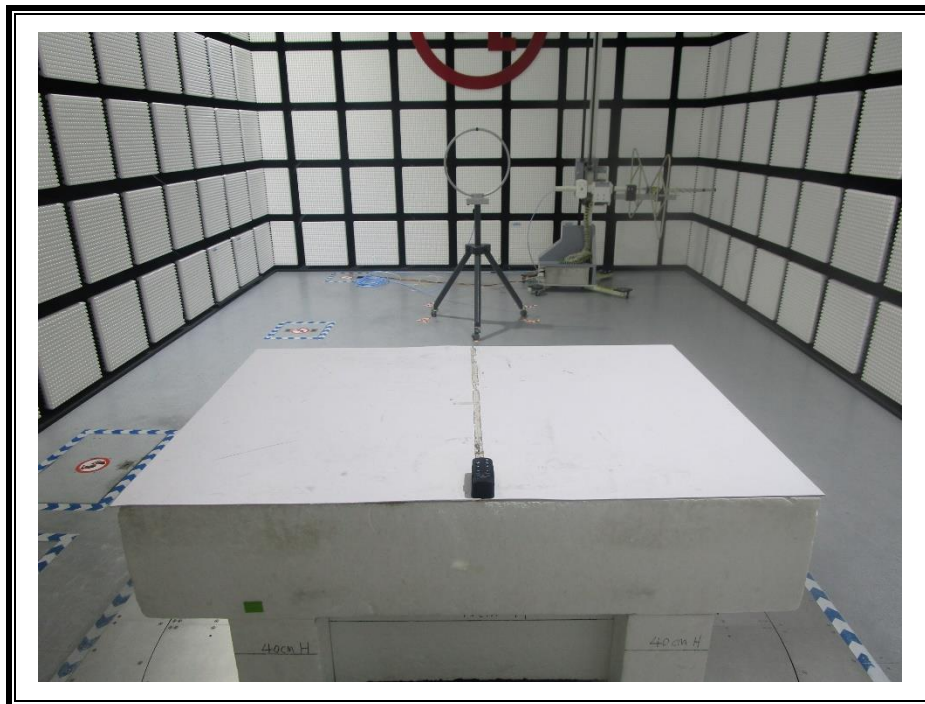
RADIATED RF MEASUREMENT SETUP (Below 30MHz)
