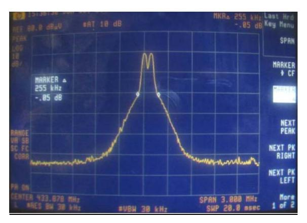
Plot of the Transmitter Bandwidth Measurement
