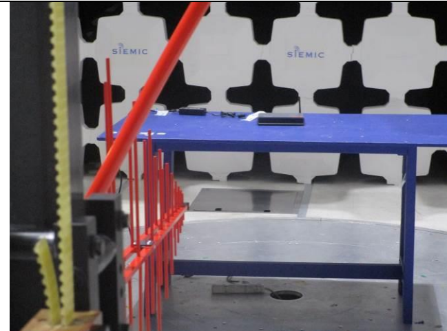
Radiated Emission Test setup (<1GHz) – Front View
