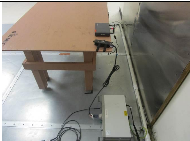
Conducted Emission Test setup – Rear View
