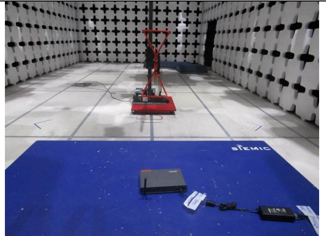
Radiated Emission Test setup (<1GHz) – Rear View
